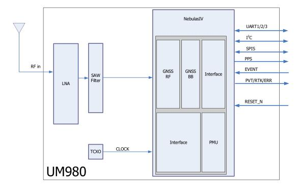
Figure 1-2 UM980 Block Diagram
