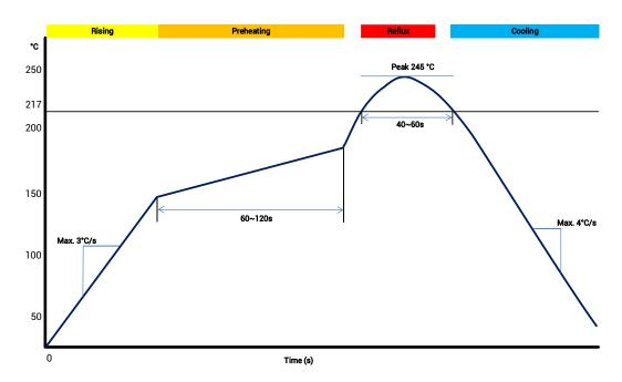
Figure 4-1 Soldering Temperature (Lead-free)
