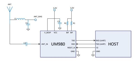
Figure 3-1 Recommended Minimal Design
