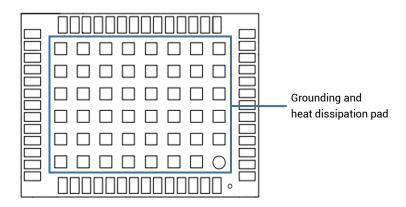
Figure 3-3 Grounding and Heat Dissipation Pad (Bottom View)
