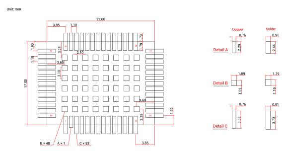
Figure 3-4 Recommended PCB Package Design
